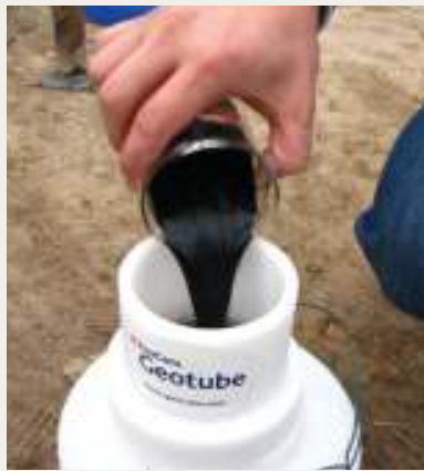
RDT test setup.
