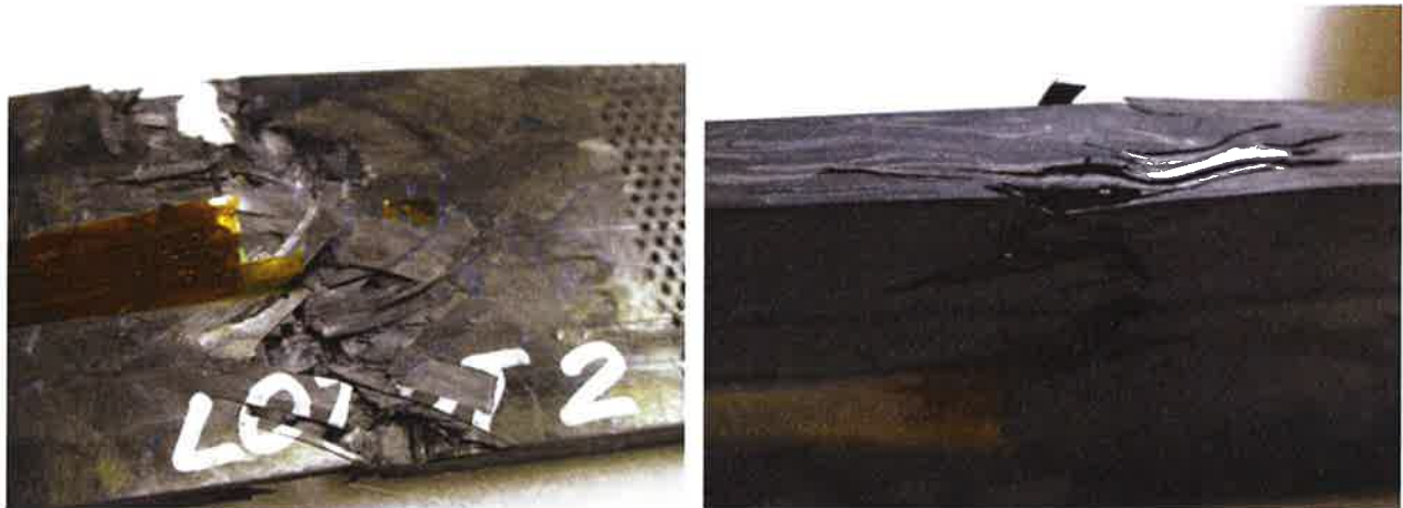
Figure 6. Tensile coupon failure modes.
