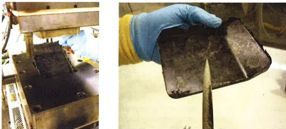
Figure 11. Demolding and deflash.
