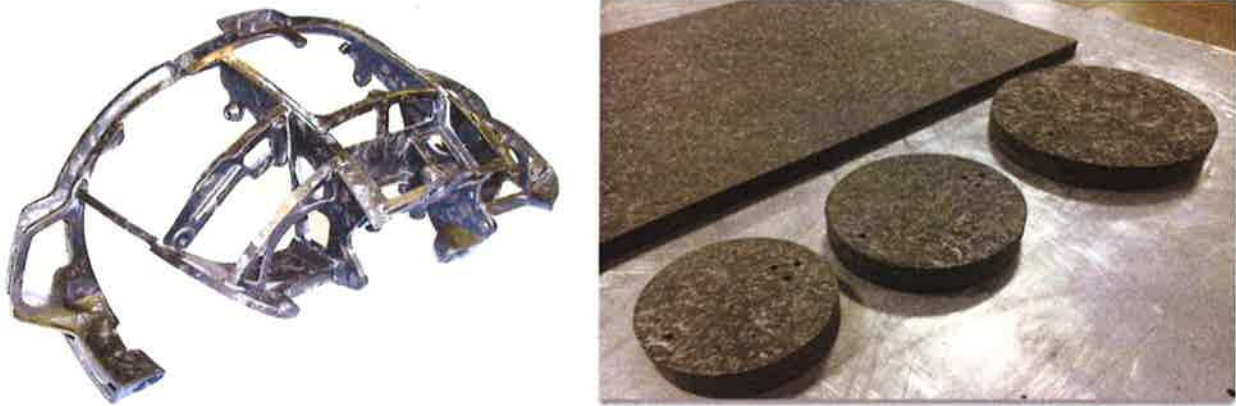
Figure 2. Helmet optical support structure and billet hard-points.
