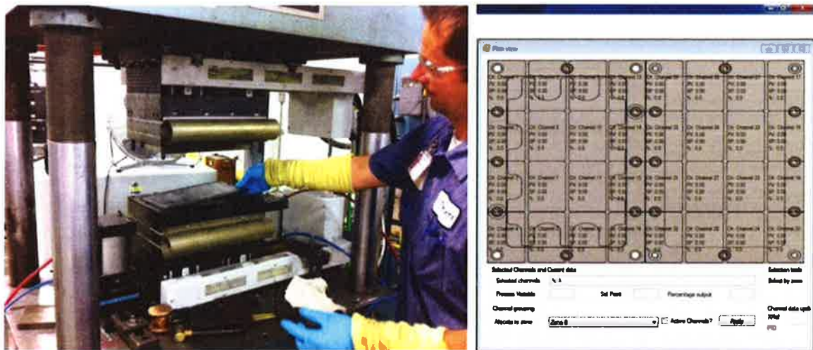
Figure 7. XPress tooling setup and heating zones.
