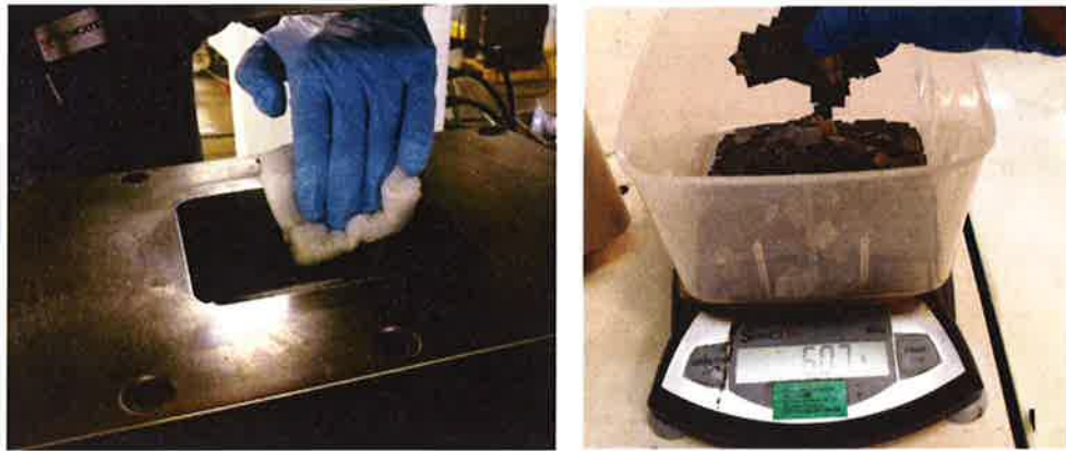
Figure 9. Mold prep and BMC weight setting.
