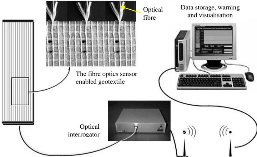
Figure 1. The TenCate GeoDetect® system components
