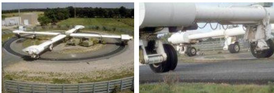
*Figure 6.* The IFSTTAR Accelerated Pavement Test facility
