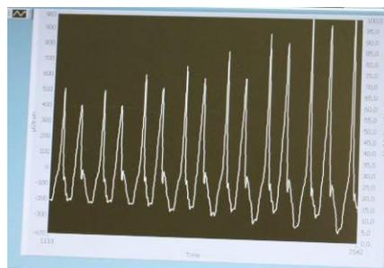
Figure 4. The strain curve measured during compaction with an increasing strength. The peaks corresponding to the passes are visible.
