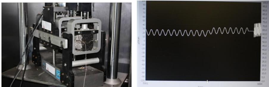
*Figure 5.* The specimen beam inside the four points bending machine (left) and the strain curve resulting of sinusoidal bending cycles producing strain variation of 10 micro strains amplitude (right).
