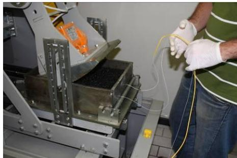
Figure 3. Compaction of the second layer of bituminous concrete.
