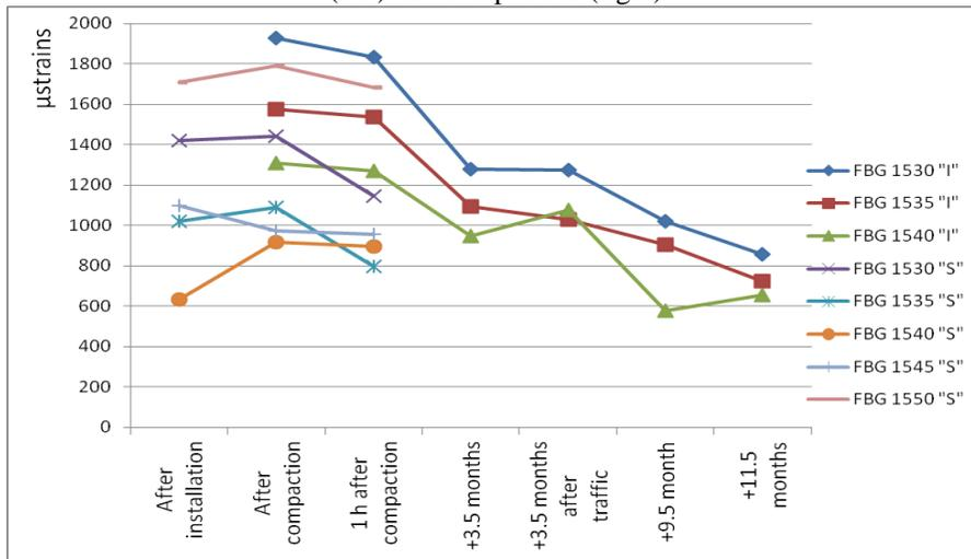
Figure 8. Relative strain measured by the Fibre Bragg Gratings during and after installation in the asphalt pavement. Zero value: just before installation.
