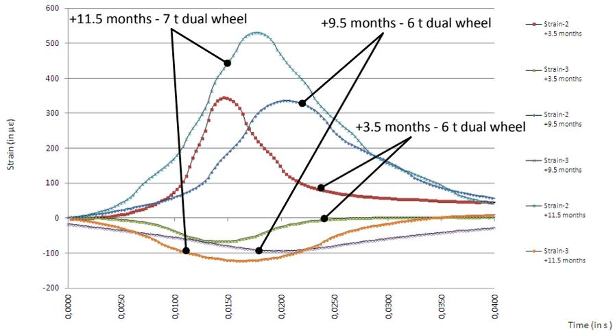
Figure 10. Strain curves measured with the fibre optics sensor enabled geotextile resp. +3.5, + 9.5 and 11.5 months after installation.
