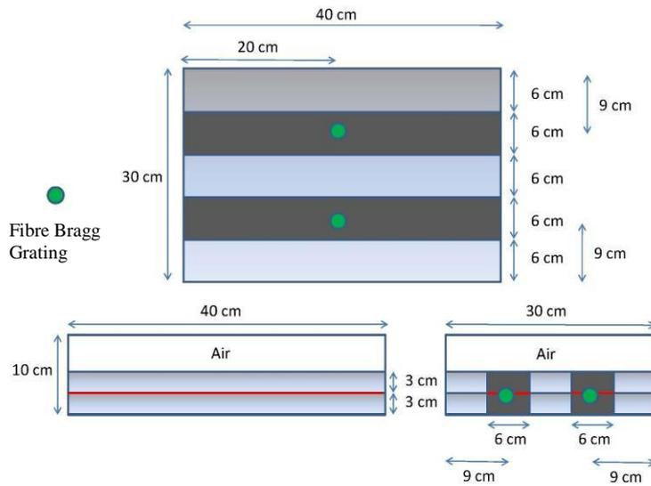
Figure 2. Top view (above) and cross-section of the concrete asphalt blocks preparation, each producing two specimen beams with one strip of sensor enabled geotextile (red) embedding one optical line and one Fibre Bragg Grating in the middle of the beam.
