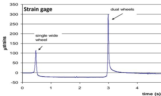
Figure 9. Comparison of the transverse strain measured at the base of the bituminous layer under the 4 rolling wheels with the fibre optics sensor enabled geotextile (+3.5 months) and strain gages
