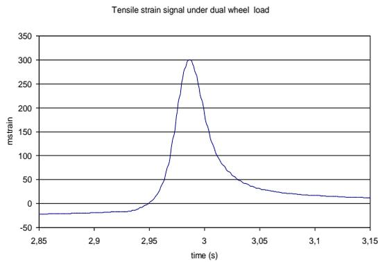
Figure 11. Strain curve measured with strain gages
