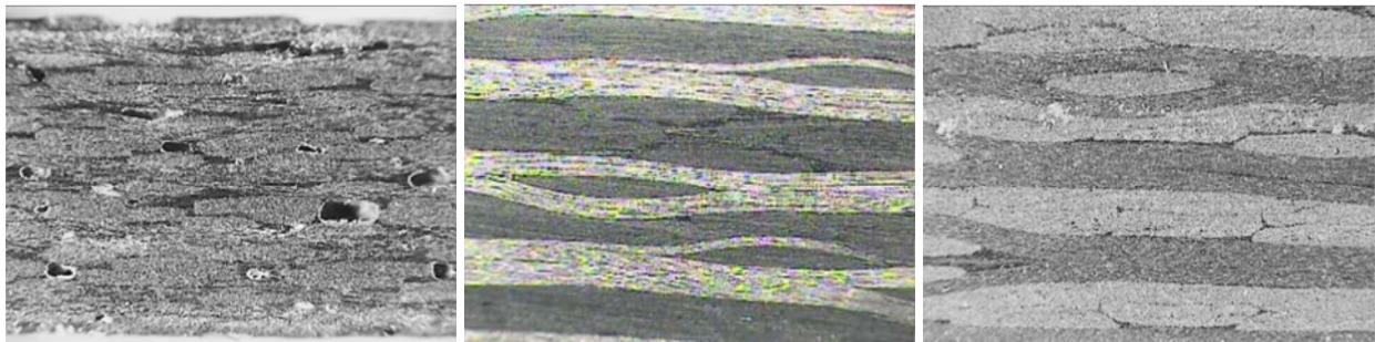
**Figure 10:** Optical micrographs (left to right) of (i) a low-quality S-2 glass laminate, (ii) a high-quality T650-35 laminate prior to thermo-oxidative aging, and (iii) T650-35 laminate cross-section after aging for 100 h at 316°C.
