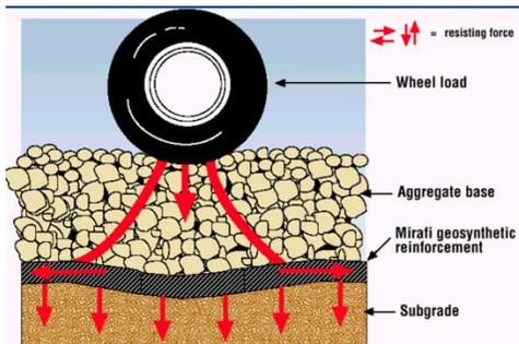
Geosynthetic stabilization and reinforcement is a mechanical process. The geosynthetic is placed within the subgrade or subbase and works with the soil and stone to create a reinforced section through separation, confinement and/or reinforcement.
