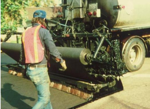
Figure 5: Distributor mounted equipment
