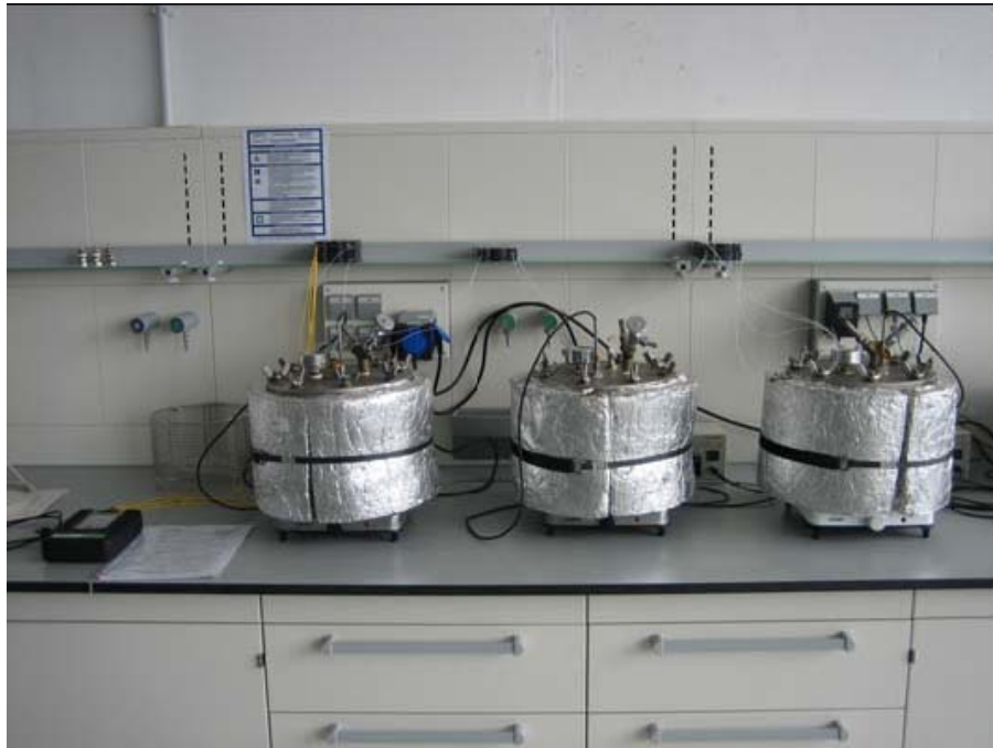
Figure 9. Test set-up at SKZ: three autoclaves with optical fibers (filled with salt water and heated at 70°C,80°C and 90°C) respectively.
