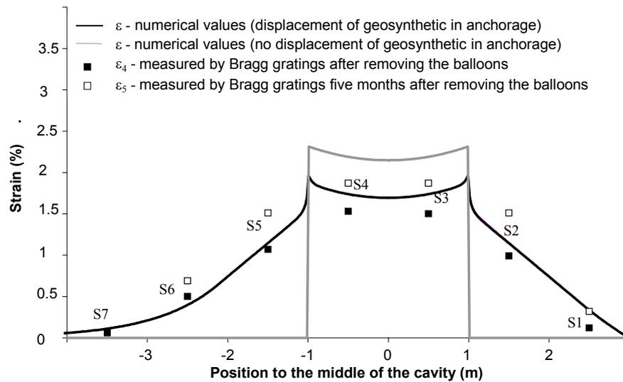
Fig. 5. Comparison of geosynthetic strain calculated and measured by the Bragg gratings
