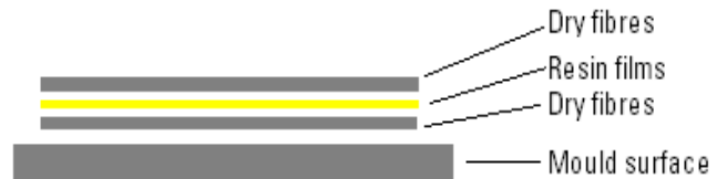
Schematic of 1 ply of Rapi-Ply
