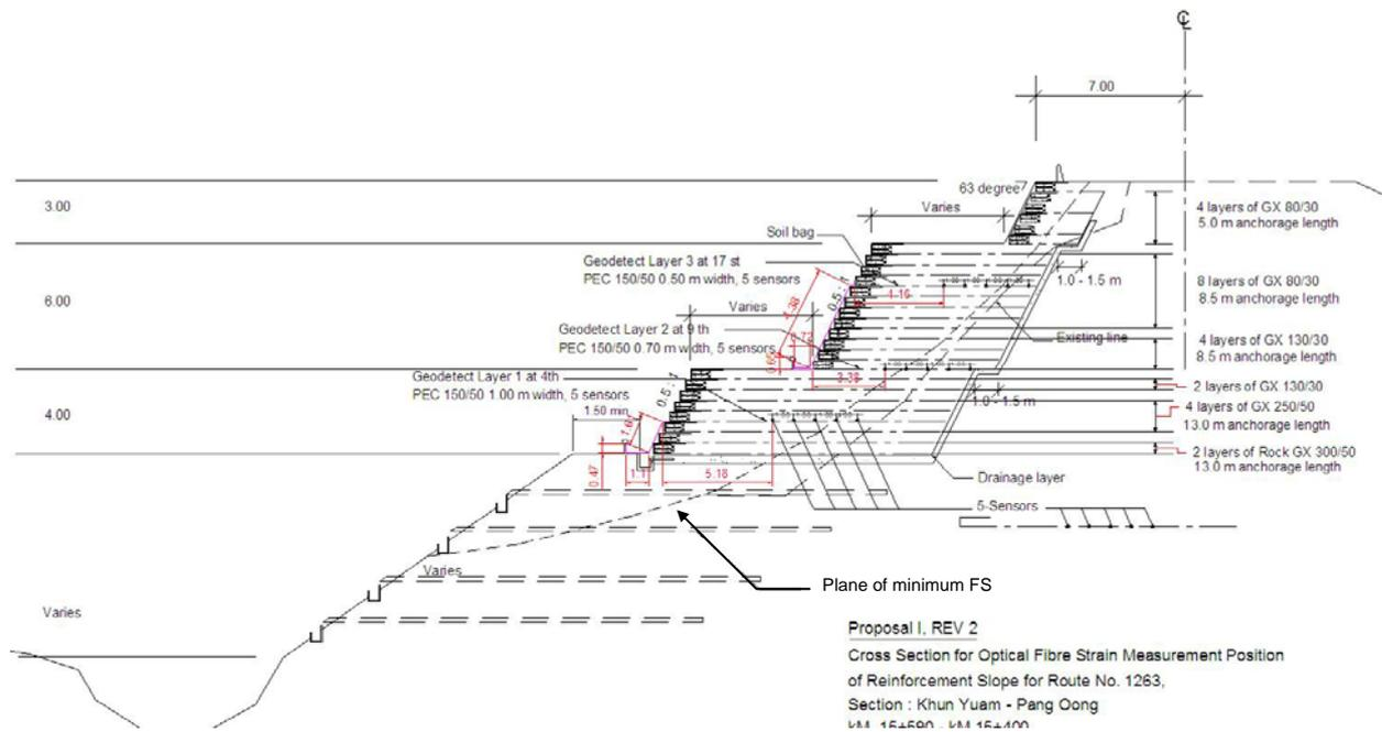
Figure 5. Typical cross section of the reinforced slope and the location of the fibre optic strain sensors.
