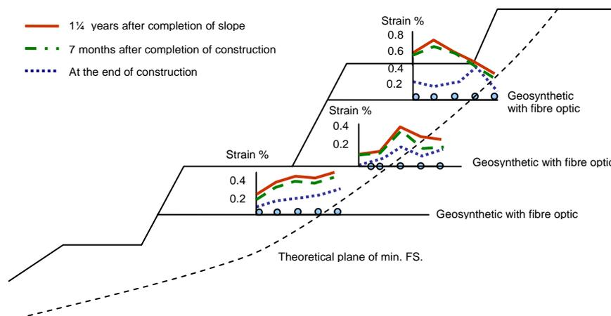
Figure 6. Strain measurements along the geosynthetic reinforcement.
