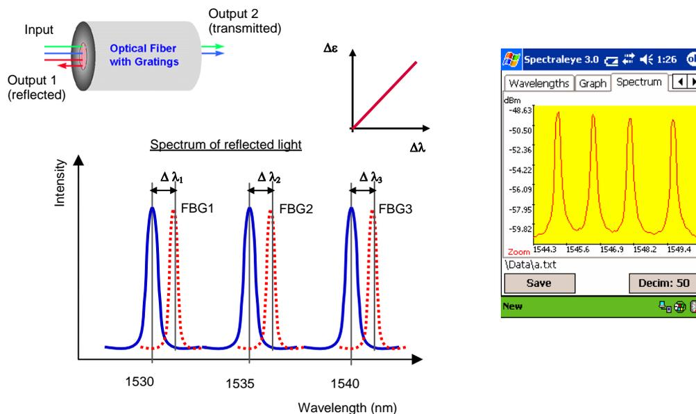
Figure 1. Principle of Fibre Bragg Grating (FBG) sensors.
