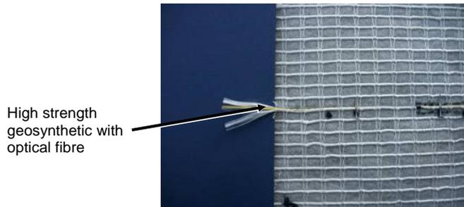
Figure 2. 'Intelligent' geosynthetic with optical fibre inserted into a reinforcing geosynthetic through a special manufacturing process.
