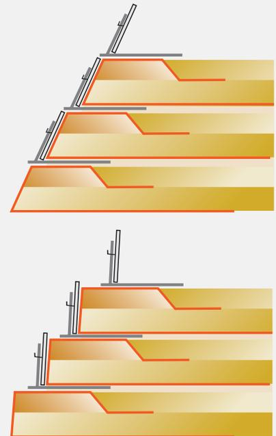
Construction of slopes by means of inclined steel angles (top) or by stepped constructing (below).
