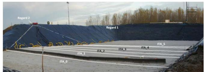
Figure 9: Location of the 6 GeoDetect® strips into the sand below the IJkdijk experimental dike.
