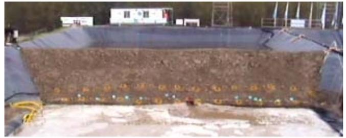
Figure 8: Downstream side of the IJkdijk experimental dyke a few minutes before collapse with clear view of the piping channel and sand erosion at the toe. The coloured labels at the toe indicate the observed flows, red with sand transport, blue only water (from Stichting IJkdijk).
