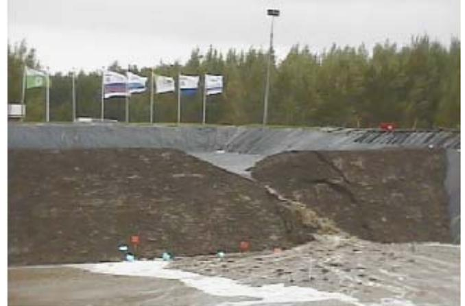
Figure 13: Collapse of the IJkdijk-Piping experimental dyke after the internal erosion process is completed (from Sticing IJkdijk).
