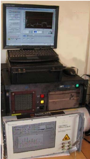
Figure 2: The Raman instrumentation for temperature measurement (on top) and the Brillouin instrumentation for strain measurement (at the bottom)
