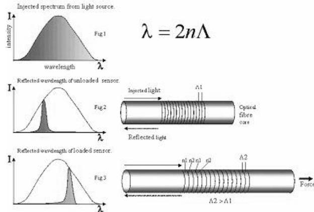
**Figure 1. FBG response as function of strain**
