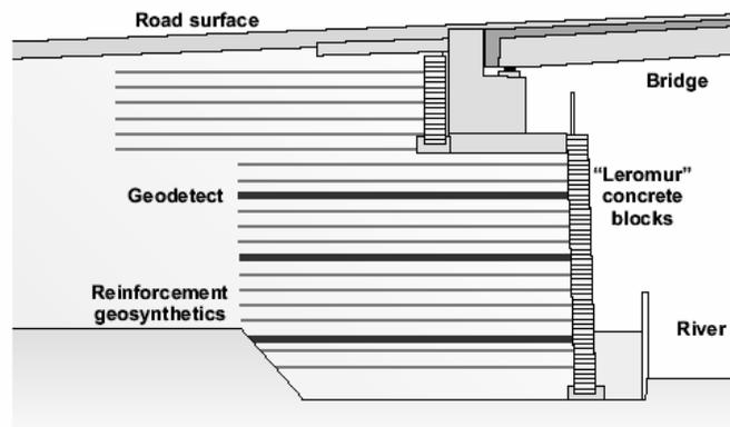
**Figure 2. Distribution of strips within the northern abutment**
