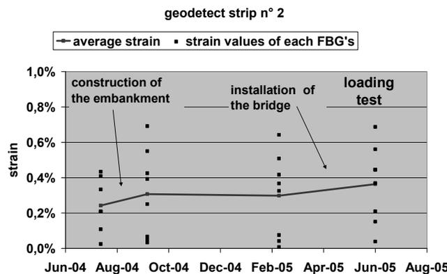
**Figure 5. Evolution of strains measured on strip n°2 during construction.**
