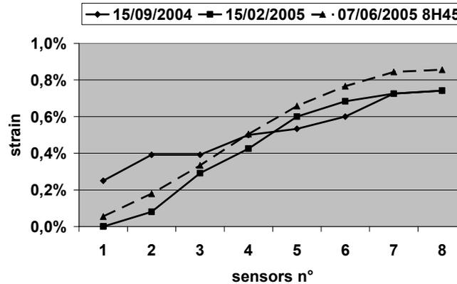
Figure 6: Strain profiles of strip No. 1 at different times
