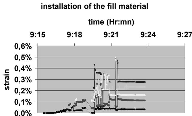
**Figure 4. Measurement during installation of strip No. 1**
