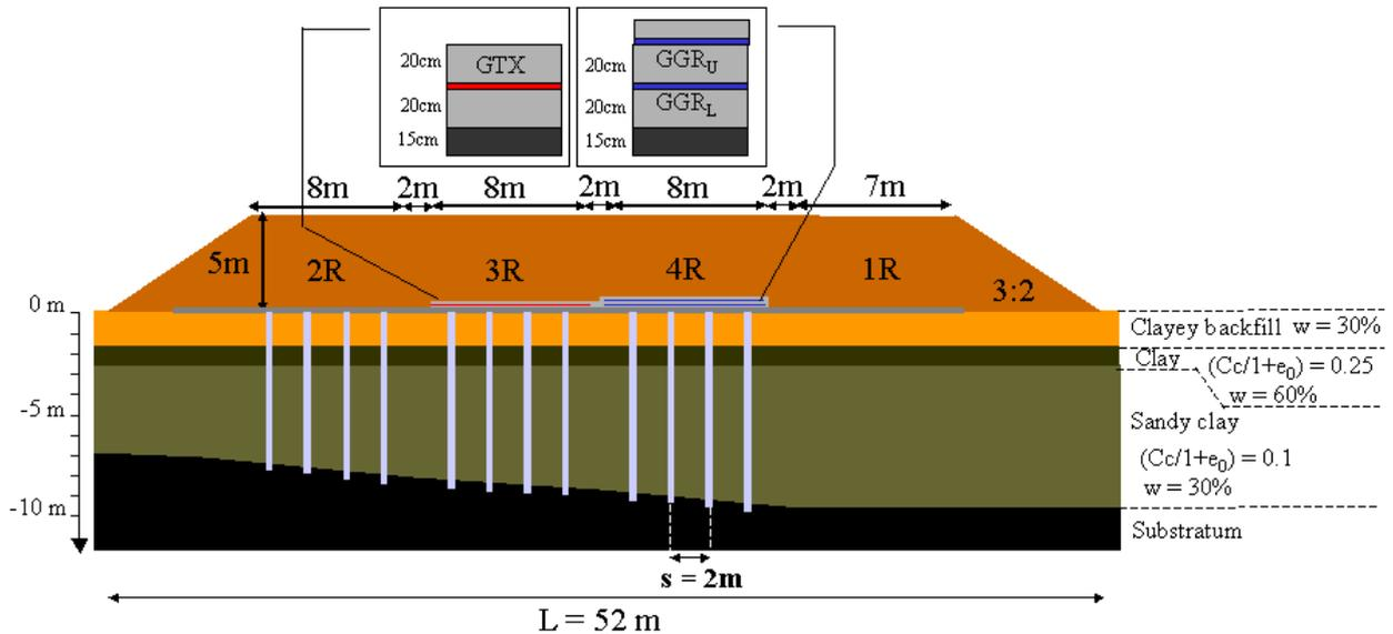
Figure 1. Typical site cross-section and geometrical characteristics
