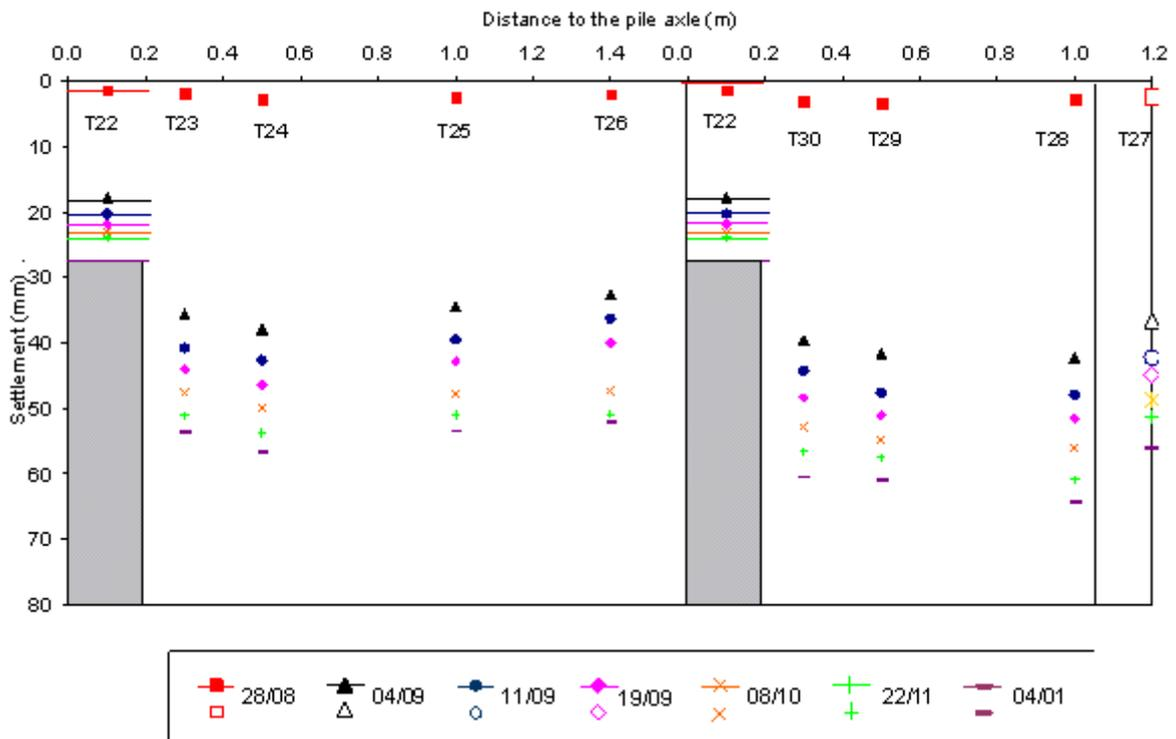
Figure 6. Settlement in section 4R
