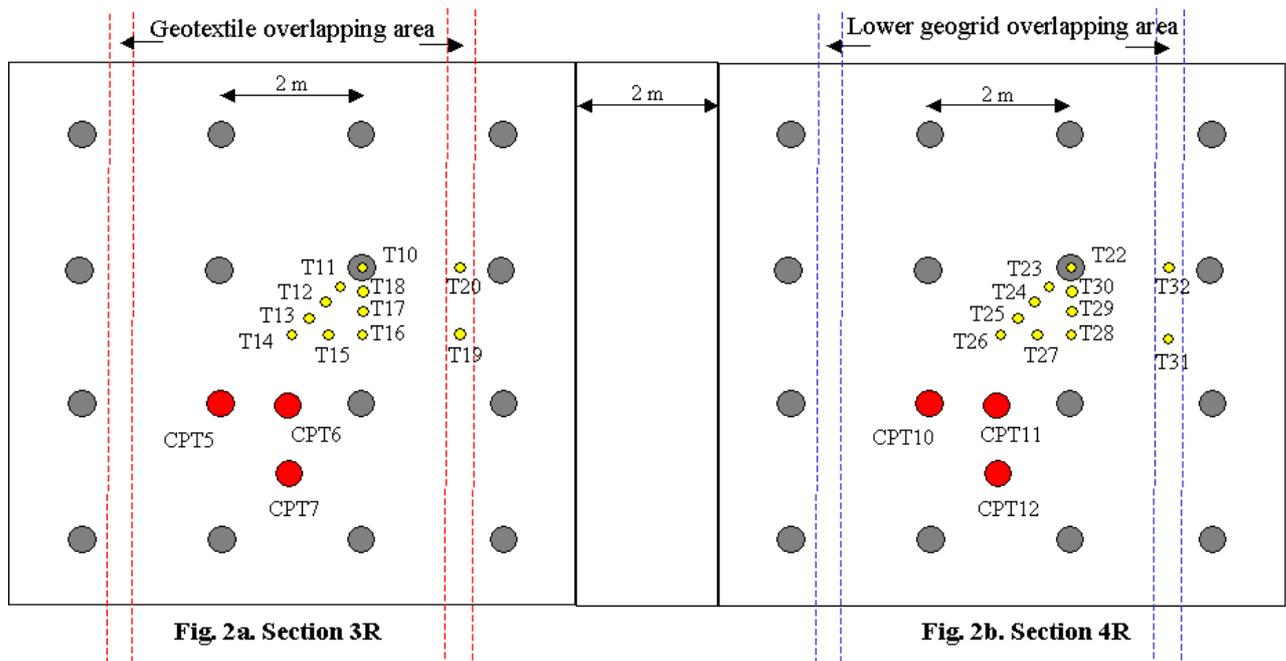
Figure 2. Instrumentation of sections 3R and 4R at the pile head level
