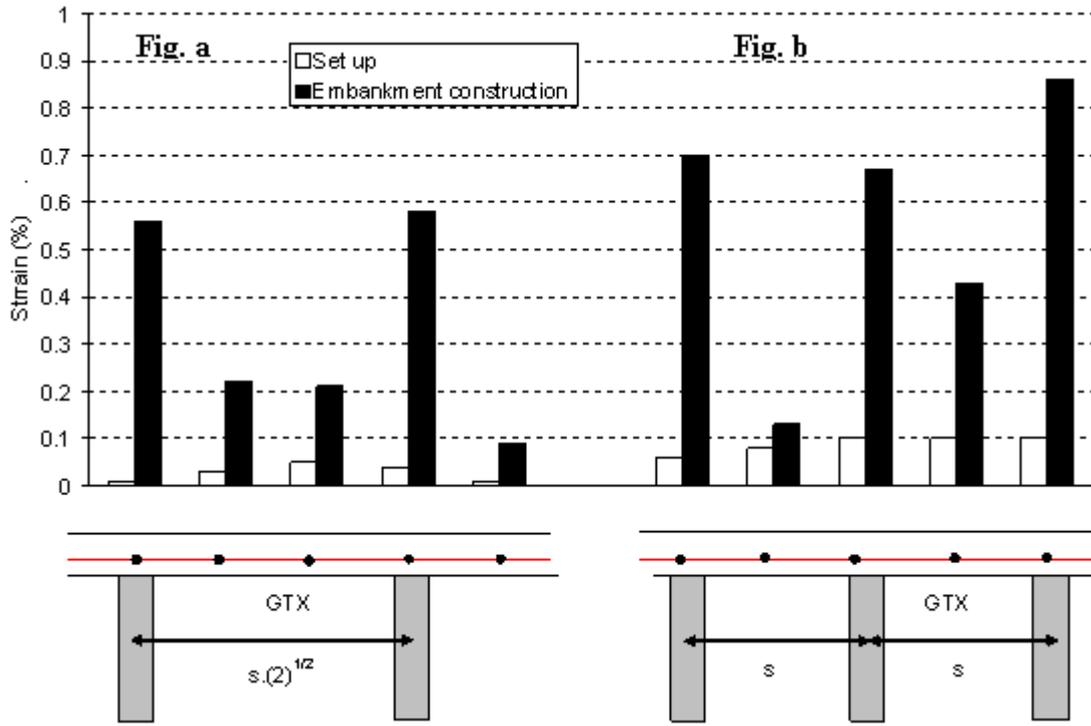
Figure 8. Geotextile strain
