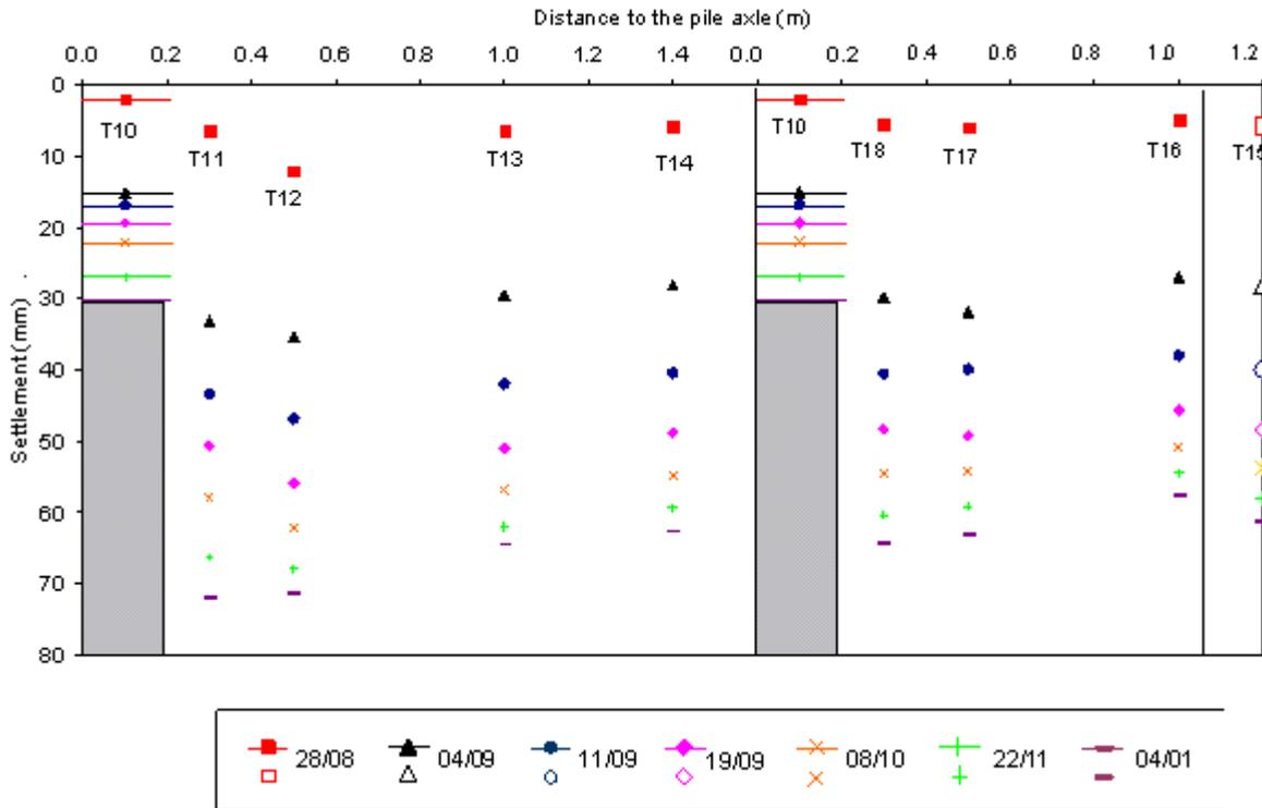
Figure 4. Settlement in section 3R
