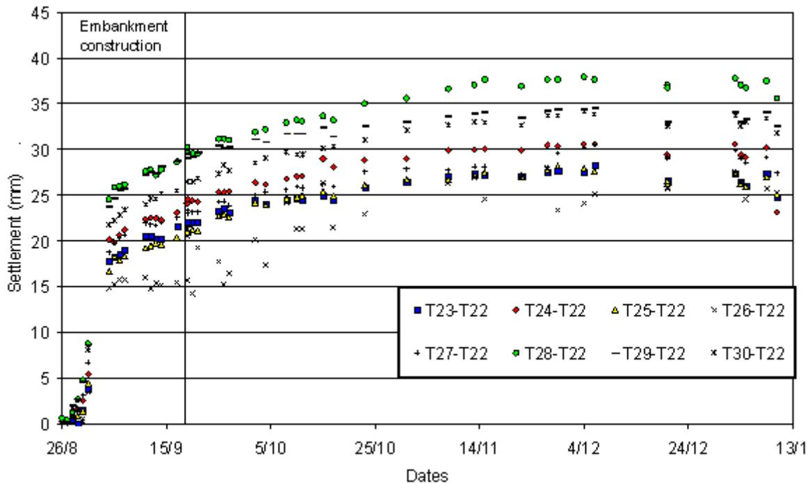
**Figure 7.** Differential settlement in section 4R
