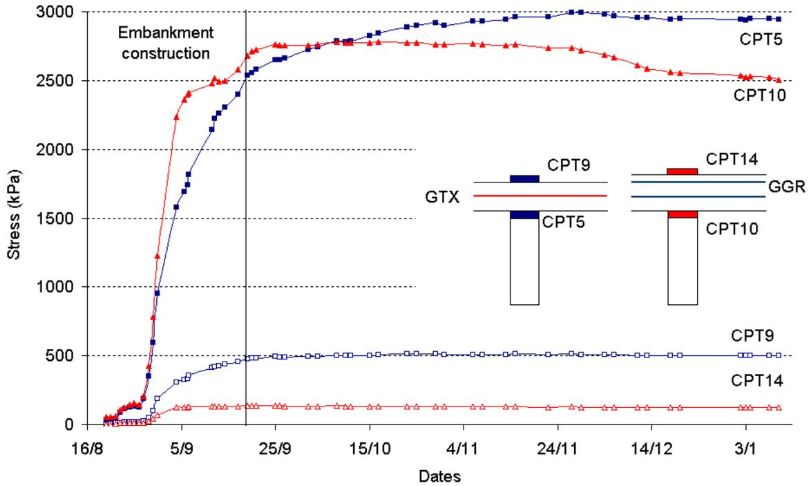
Figure 3. Load transfer measurement (stress on pile)
