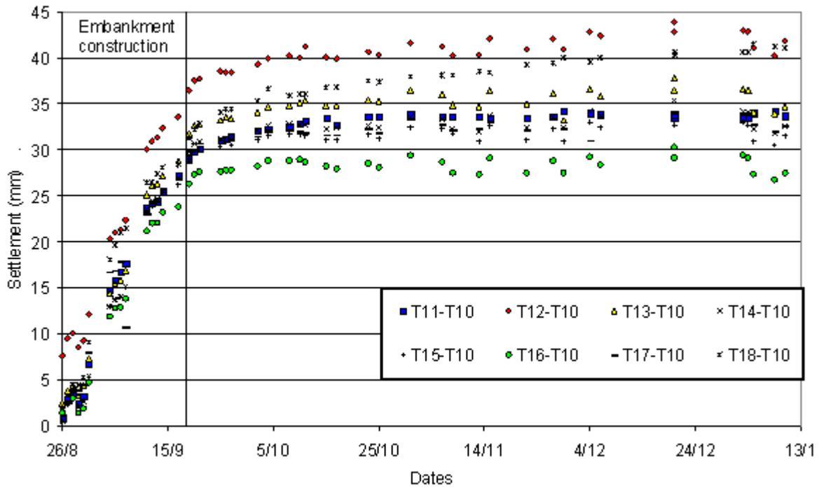
Figure 5. Differential settlement in section 3R
