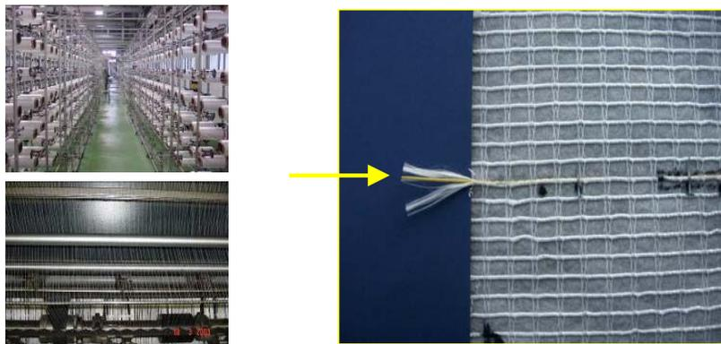
Figure 4. Optical fiber inserted during production.
