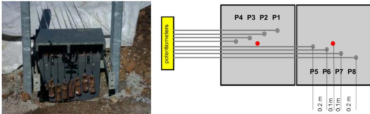
Figure 6. Measurement devices (extensometers) complementary to the Invar wire and potentiometers.
