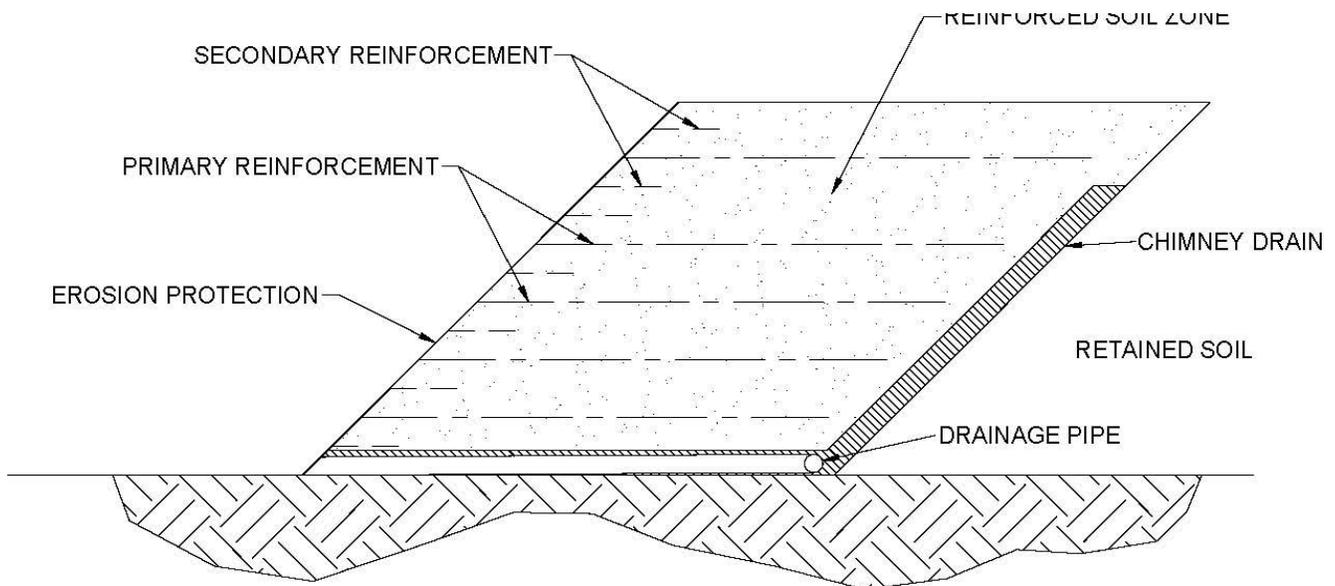
**Figure 1. General Cross-Section of a Reinforced Slope System**
