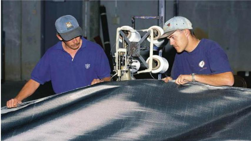
**Figure 4. Factory Sewing with double-needle machine**
