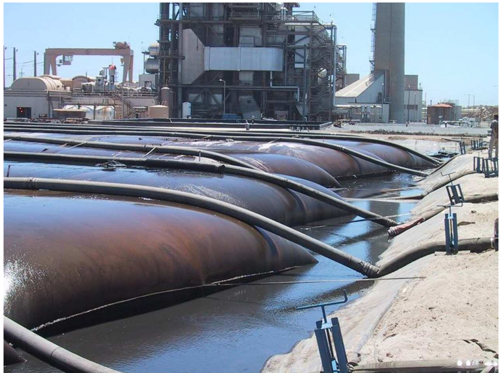
Geotube® dewatering technology in use. Water drains from the specially designed fabric bags, while the solids are trapped behind, making removal and recovery simple and cost effective.
