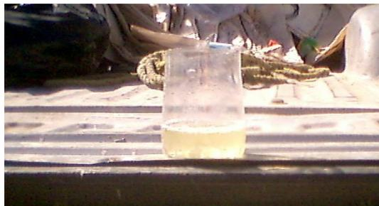
*Effluent analysis showed more than 95% of solids removed.*
