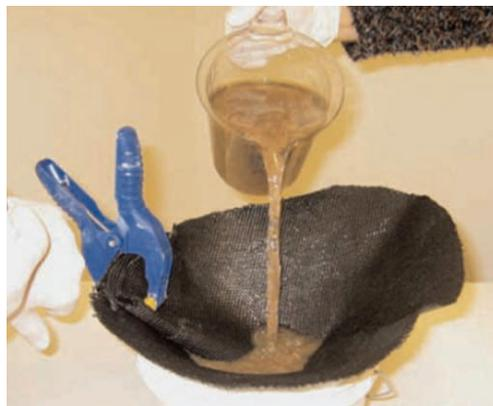
The Cone Test provides information similar to the RDT. It requires only a sample of Geotube® dewatering fabric fashioned into a cone.
