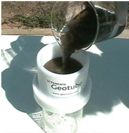
version of the test can be conducted with just a sample of Geotube® GT 500 material. **The Cone Test** provides the same information as the RDT, using only a piece of Geotube® material fashioned into the shape of a cone to catch the sludge and allow it to drain into a container.
