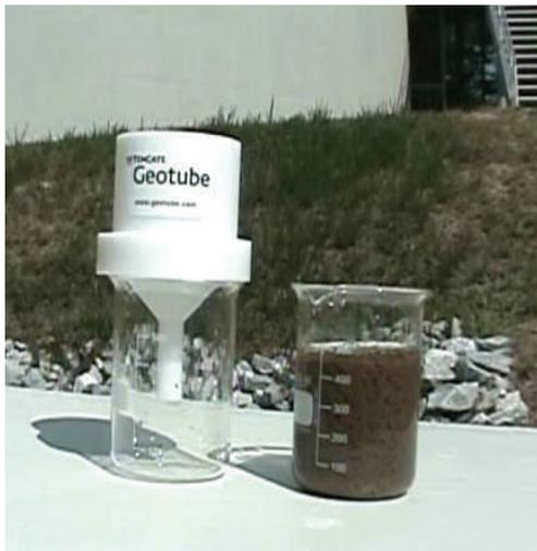
The Geotube® Rapid Dewatering Test (RDT) uses a specially designed funnel. A disc of Geotube® fabric is placed in the bottom, and the sludge filters through it. The RDT can quickly provide a basic evaluation of how well a material can dewater. It is also very useful for assessing different polymer treatments.
