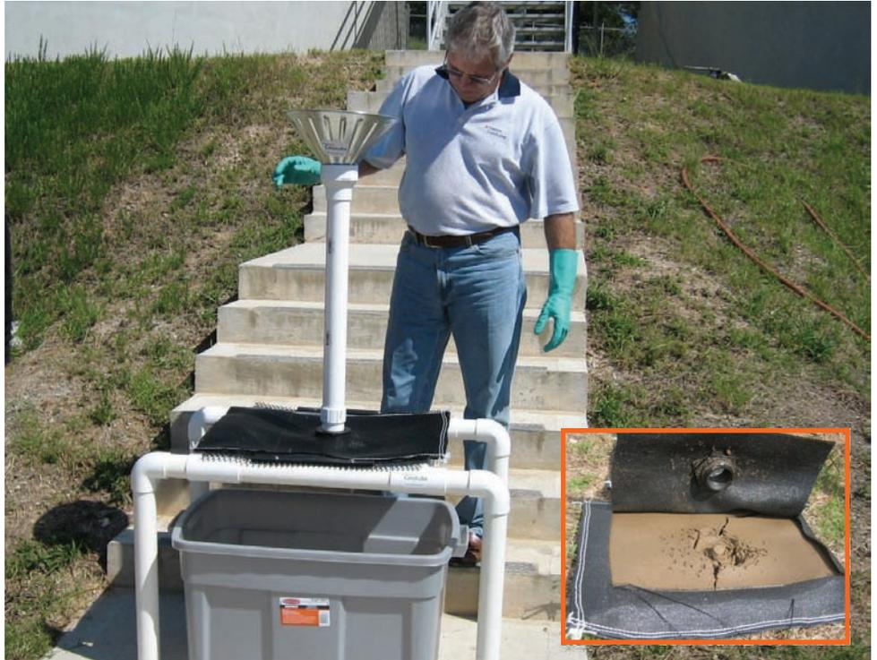
*The Geotube® Dewatering Test (GDT) is a simplified field-scale test designed to replace the former Hanging Bag test. A one cubic foot Geotube® container is used to test dewatering efficiency for different sludge samples. Results accurately predict full-scale Geotube® dewatering operation. The container can be cut open and the dewatered sludge tested further (see inset).*
