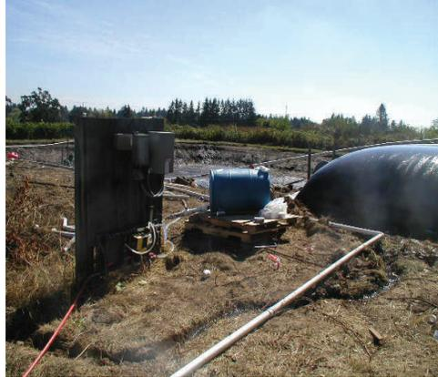
Figure 2. Polymer metering system with Geotube® unit.
