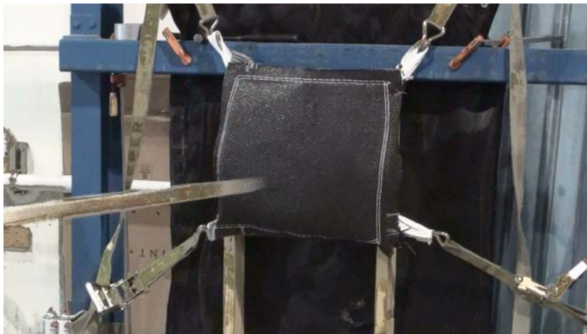
Impact testing conducted per the large missile impact test requirements of ASTM E1886/E1996.
