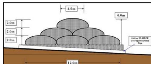
*Above: Cross section of the upper Geotube® debris dam. Below: Drainage raceways lead into the tailings lagoon area prior to the Geotube® debris dam installations.*
