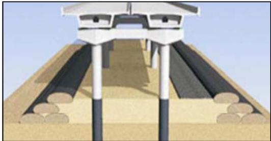
This illustration shows a cross section of the Geotube® bridge platform design for the artificial island.
