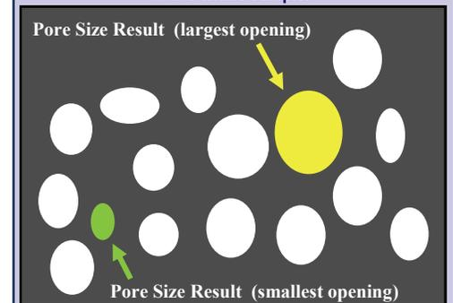
**Typical Results from Capillary Flow Pore Size Testing**
