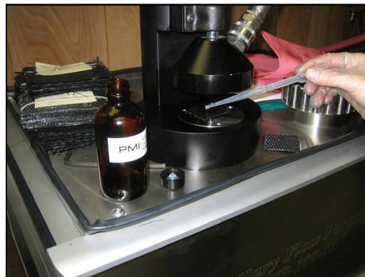
Sample being prepared for testing in porometer.
