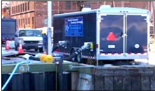
*Silt concentrations were required to be regulated and maintained accordingly for this project. The SmartFeed® patented mobile chemical feed system provided automated polymer mixing injection to the silt prior to it reaching the Geotube® units in the anchored barges.*
