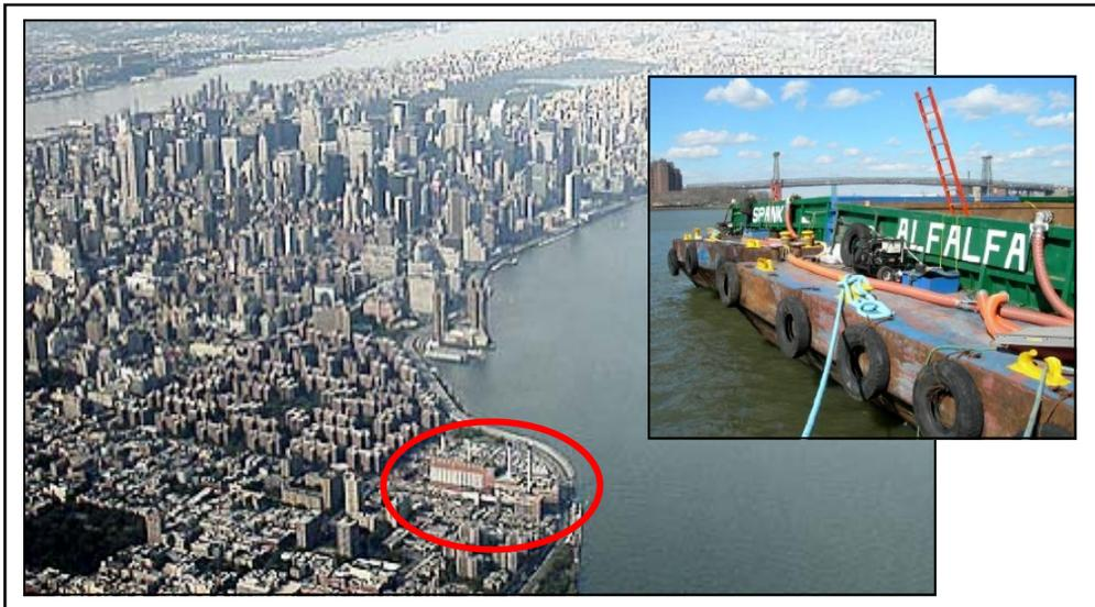
*This aerial photo of New York City shows the crowded landscape of the power generation plant. For this innovative dewatering operation, Geotube® units were installed in two floating barges on the East River (inset photo).*
