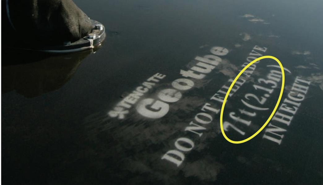
*Maximum allowed pumping height is printed on every Geotube® unit. Do not exceed.*
