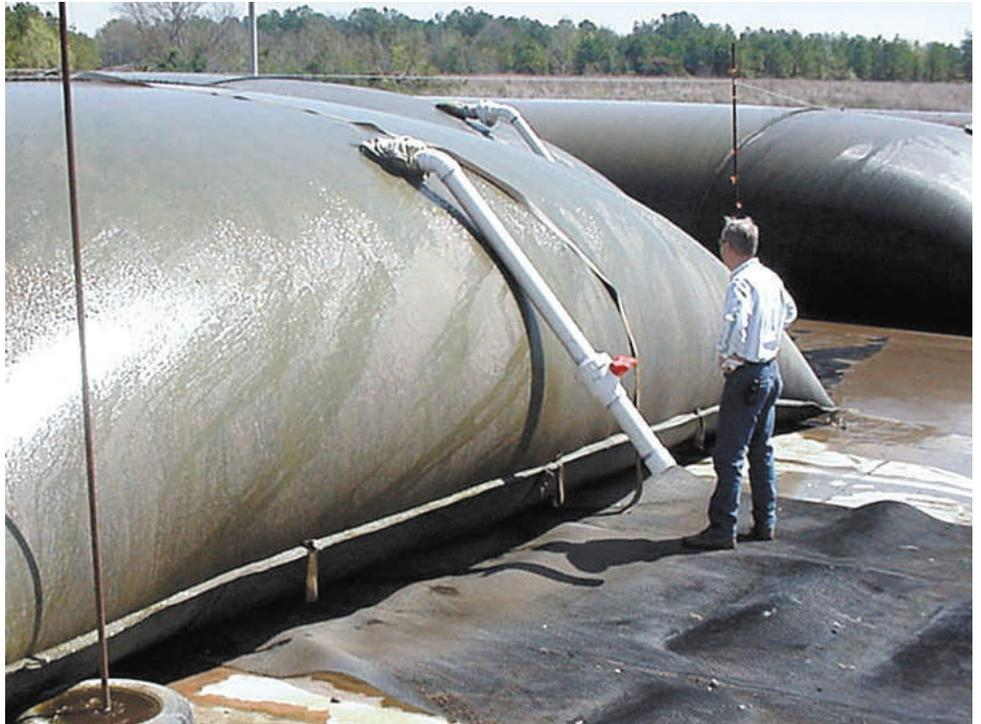
*Geotube® units are constructed using exceptionally strong fabric and patented seaming techniques. The result is a product that allows for pumping heights greater than any other product on the market. This allows for extra capacity and faster dewatering.*
