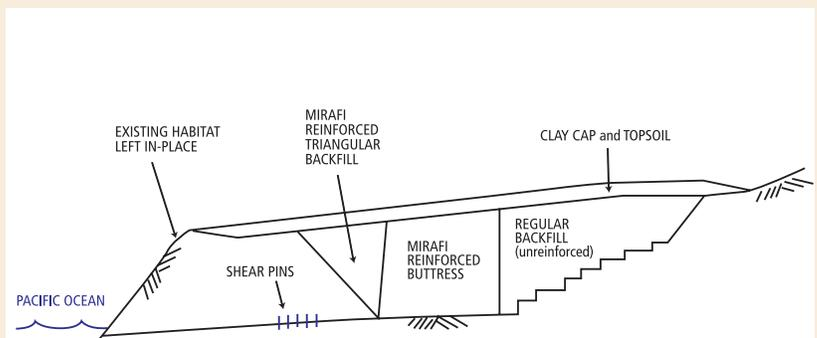
**Figure 1.** Cross-sectional drawing of the reinforcement strategy.
