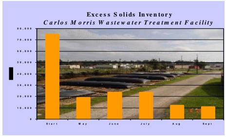
Figure 3. The plant operators have been able to reduce their solids inventory by using Geotube® dewatering containers.
