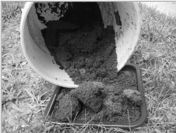
After dewatering with Geotube® containers, cake solids were at 54%.
