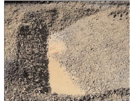
Wet, soft subgrade exposed in the test pit.
