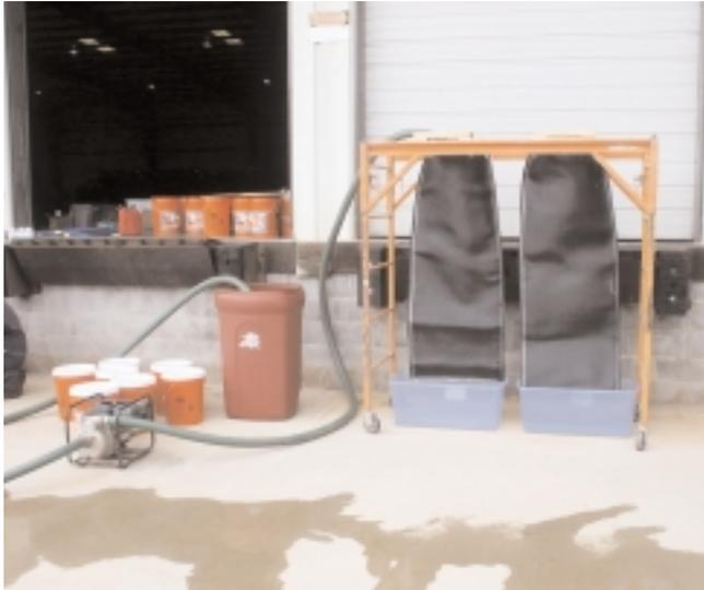
**Step 1: Conduct a Geotube® Hanging Bag Test**
