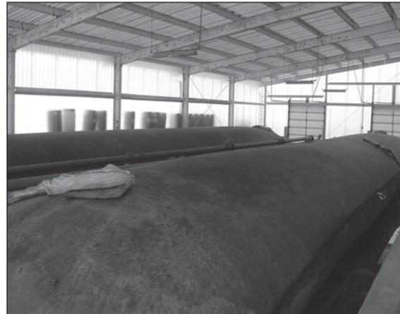
Geotube® containers took one load each day, whereas a drying bed required 3 days to dewater.
