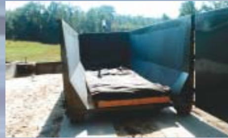
The Geotube® MDS™ unit folds out into a roll-off container.
