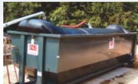
Geotube® MDS™ can be pumped several feet high for maximum volume.
