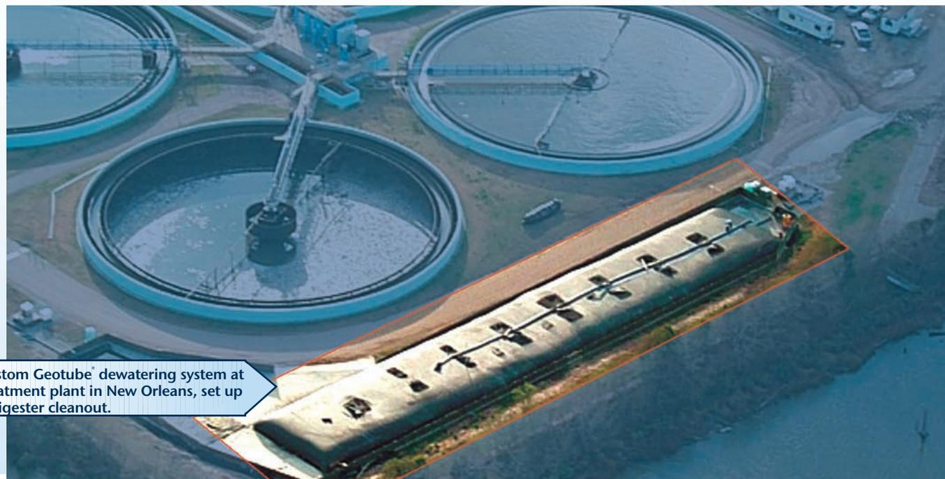
A custom Geotube® dewatering system at a treatment plant in New Orleans, set up for digester cleanout.
