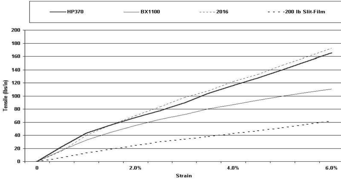
Stress-Strain Curves (0% to 6% Strain) Stress-Strain Curves (0% to 6% Strain)
