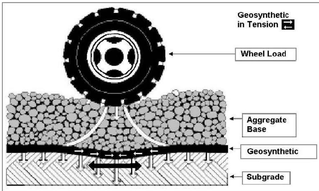
**Figure 1:**Unpaved Roadway Cross Section
