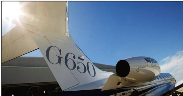
The G650's skins, ribs and spars are fabricated with TenCate's Cetex® carbon fiber reinforced thermoplastic prepreg laminates utilizing a polyphenylene thermoplastic resin. The multi-ply thermoplastic laminate ribs are press formed, and then subsequently robotically welded via induction welding. The Gulfstream G650 is targeting a 2012 in service
