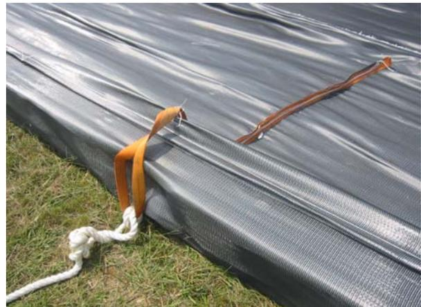
Figure 7. Polyester webbing was used for the strap to attach to the leading edge of the fabric. A 0.3 m by 0.3 m by 2.4 m long polystyrene block was sewn in a pocket along the leading edge.
