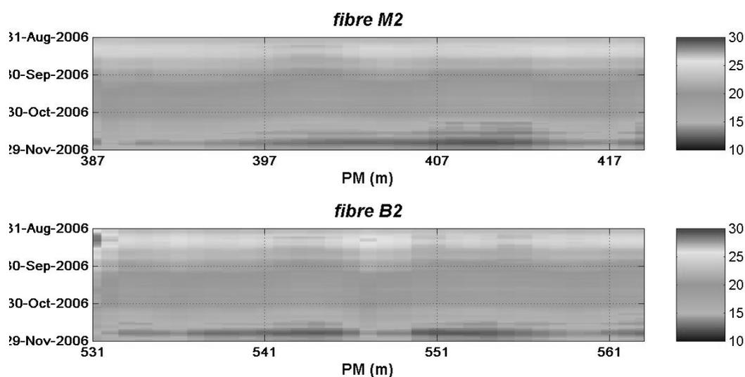
**Figure 8:** Evolution of temperatures measured along the OF – West Face
