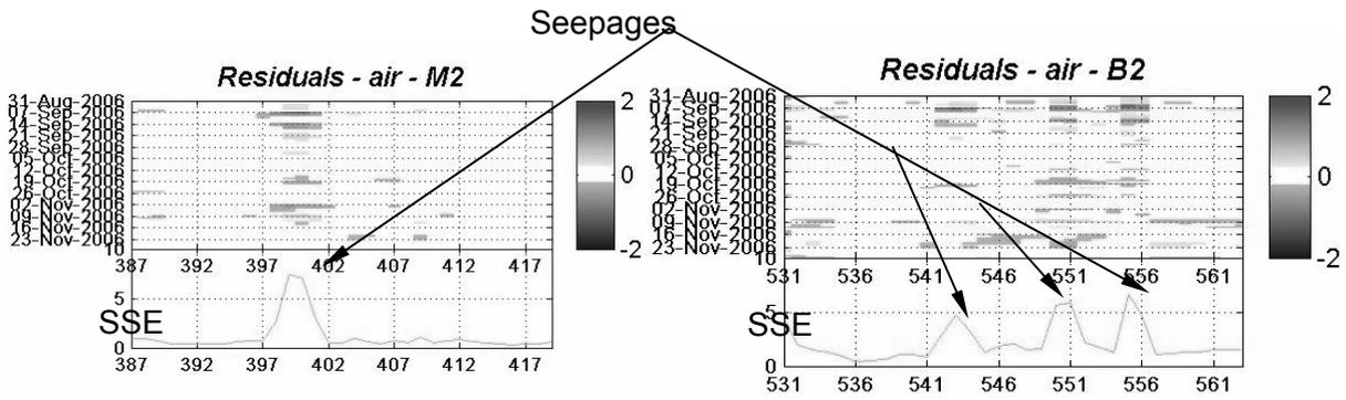
**Figure 9:** Residue after analysis and SSE – West Face
