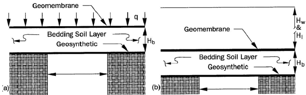
**FIGURE 11: Design Cross Sections with (a) liquid or equipment surcharge,  $q$ , and (b) soil or waste surcharge**
