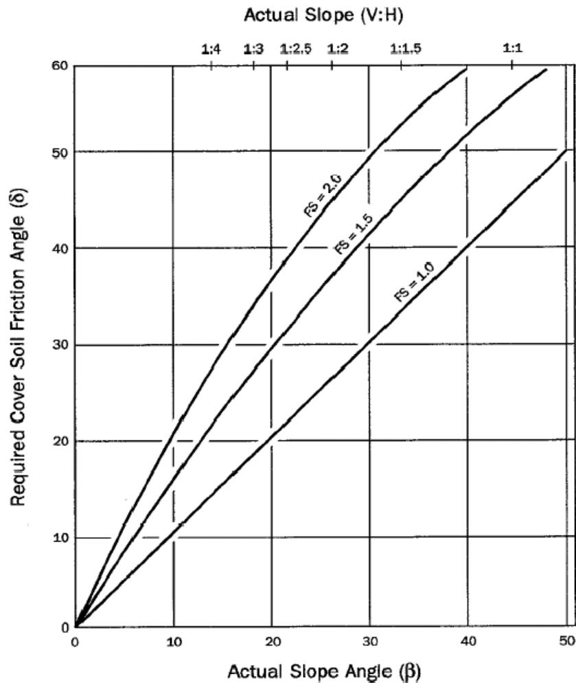
**FIGURE 6: Design Curves for Uniform Thickness Cover Soils in Geomembrane Lined Slopes<sup>(7)</sup>**
