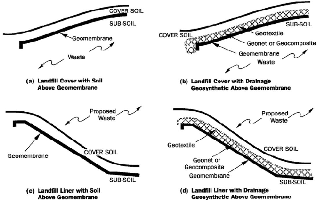
**FIGURE 4: Various Solid Waste Caps and Liners Involving Cover Soils and Geosynthetics** (after 5)
