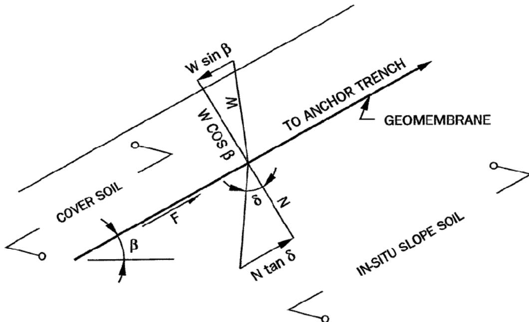
**FIGURE 5: Schematic Diagram for Force Involved with Cover Soils on Geomembrane Lined Slopes with Uniform Depth Cover Soil<sup>(7)</sup>**
