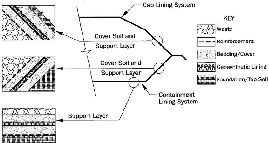
**FIGURE 3: Components of Reinforced Soil Layer Systems**
