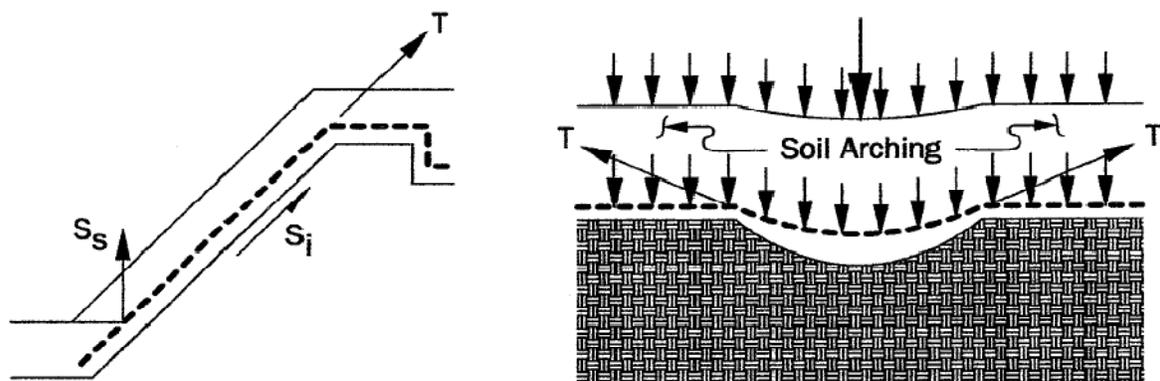
**FIGURE 2: Cover Soil Reinforcement vs. Reinforced Support Layer**
