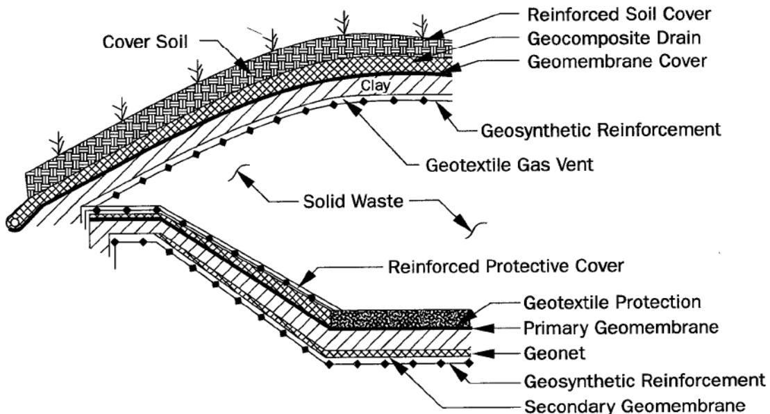
**FIGURE 1: Applications Using Reinforced Soil Layers**
