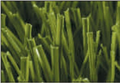
Fibres before (above) and after (below) Lisport test wear simulation of 12,200 cycles.
