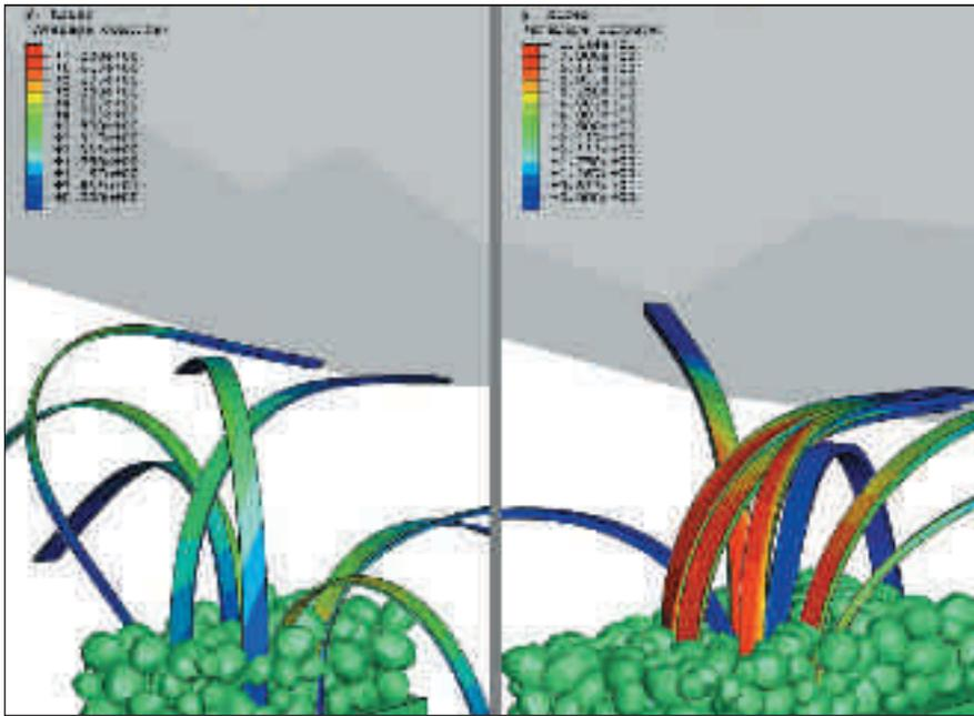
TenCate's design tool gives an animated view of what is happening 'inside' the fibre while it is exposed to force.
