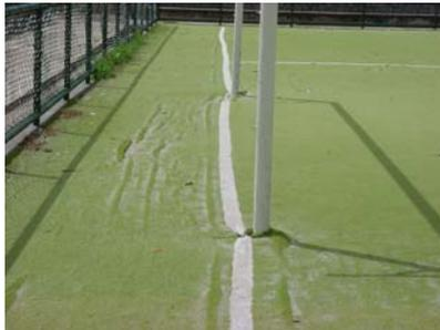
The picture shows a “growing” synthetic turf pitch. Under the influence of a constant stress the backing slowly starts to permanently deform and the carpet starts to grow. This effect is caused by viscoelastic creep in the backing.
