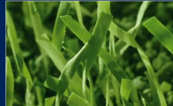
TenCate Tapeslide™ XP™ turf blades after 40,000 cycles of Lisport testing
