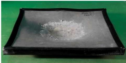
A test sample of the hull of an APC that was protected with **TenCate Armourtex BM** roadside bomb armour. The EFP is fully stopped and only an indent in the main hull is seen.
