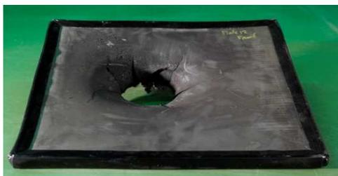
A test sample of the hull of an APC that was protected with **traditional ceramic armour** (STANAG 4569 Level 4). The EFP has perforated the main hull including a spall liner completely.
